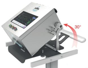
A front 7" wide TFT Touch screen display is the user interface for data entry and monitoring functions.
